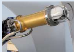
TV Camera for operations in vacuum and ultra high-vacuum environments
