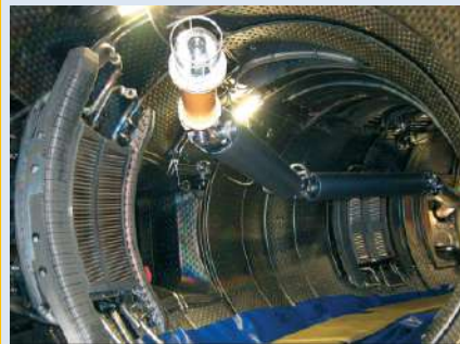
TV Camera for operations in vacuum and ultra high-vacuum environments
