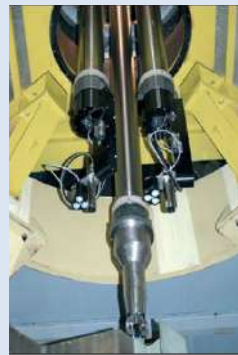
TV Camera for operations in vacuum and ultra high-vacuum environments
